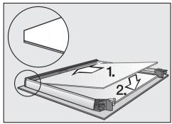
Replace the upper of the two middle panes together with the seal. The more angled corner must be at the top left.
